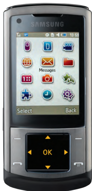
Five different options generally appear in the magical touch window. Here, when in the main menu, they're just scroll keys and OK in the middle.
