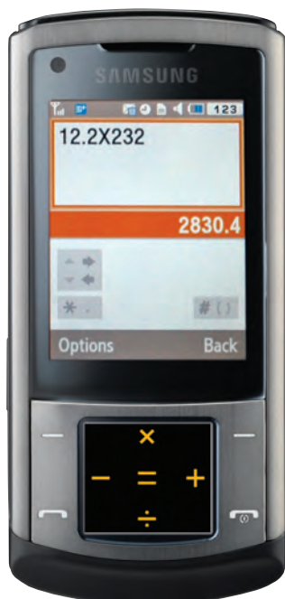
See how the magical touch window brings up calculator icons, acting as context-sensitive shortcuts, helping multiply the numbers above.
